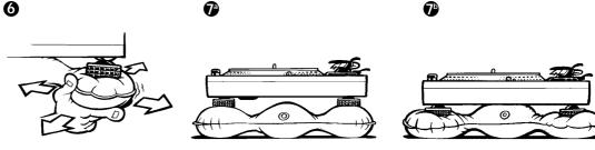
4 and points towards the DJ. In this way air can easily be expressed. Make sure that the Freefloat is unobstructed all around. Its effect decreases when it touches other 6 objects.
